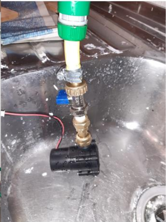
"B&Q Plumbing" and a small turbine generator
